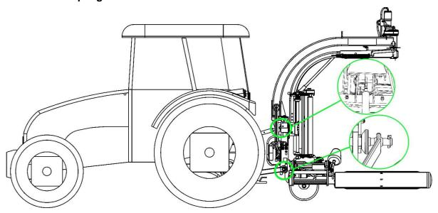
Figure 7. Point of connecting the tractor with the wrapper
