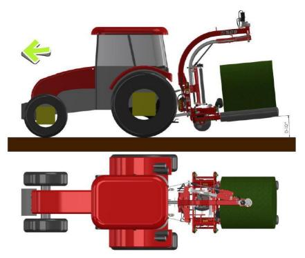
Figure 17. Position during wrapping up a bale
