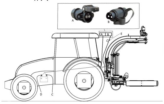
Figure 12. The connection diagram of 12 V electric power supply of the tractor to the wrapper
