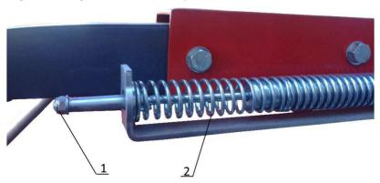
Figure 24. Spring tensioning adjustment in safety arm: 1 - nut, 2 - spring
