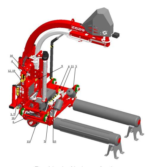
Figure 6. Location of the pictograms front view For the designations of the pictograms, see Section 1.9.
