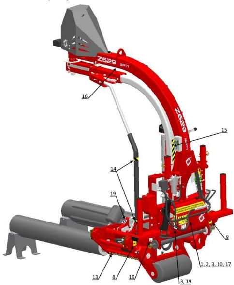
Figure 5. Location of pictograms back view For the designations of the pictograms, see Section 1.9.
