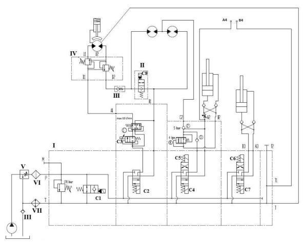
Figure 13. Hydraulic system of the wrapper:
