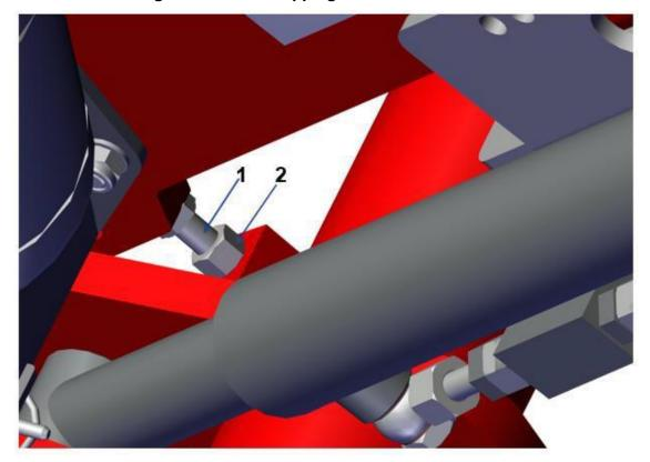
Figure 36. Limiting the arms' folding movement
