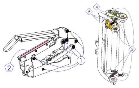
Figure 37. Lubricating points of film cutter and film feeder:
