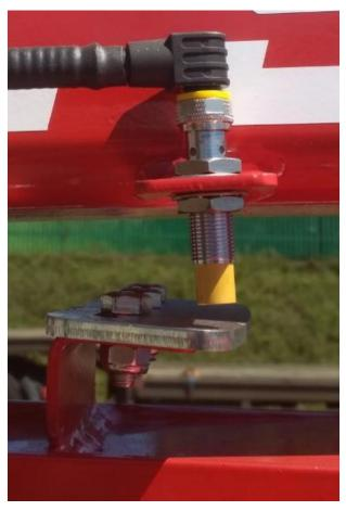
Figure 22. Inductive revolution sensor setting
