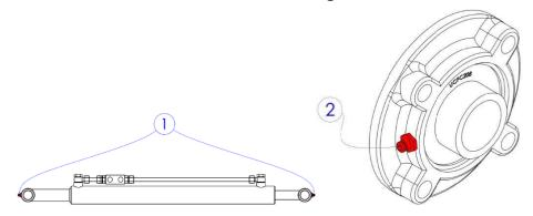
Figure 38. Lubrication point of Lower arms servomotor and bearings: 1 – pin grease nipples; 2 – bearing grease nipples
