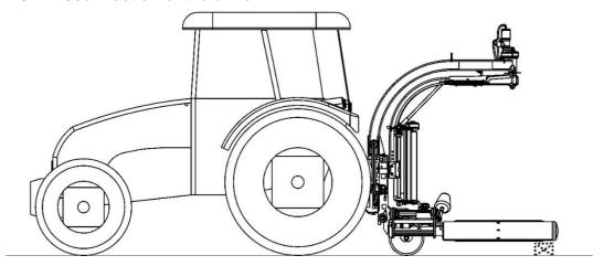
Figure 10. Wrapper position at connection and disconnection with the tractor drive
