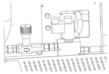
Figure 27. Non-return and throttle valve locking the tipper in the extended position
