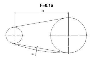
Figure 35. Chain tension
