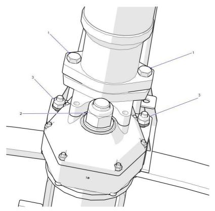
Figure 40. Transmission disassembly
