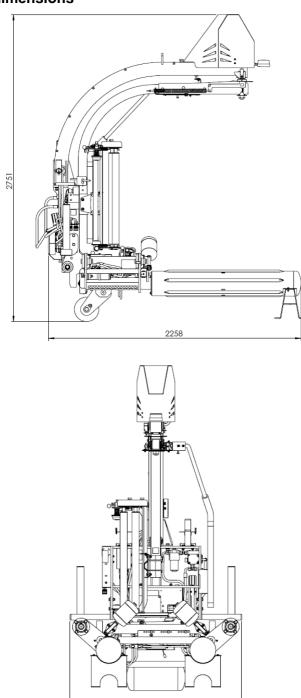
Figure 4. Overall wrapper dimensions in transport position
